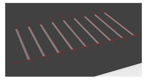
■ Paste the rail on the butyl tape, and use the plastic roller to compress the tape and rail.
